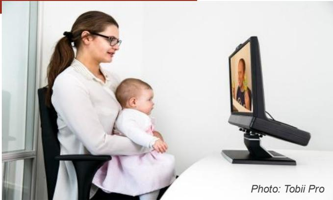
In the ELAB, we use a sophisticated, non-invasive eye tracking unit called the Tobii TX300. The eye tracker sits at the base of our monitor and follows your child's gaze and determines how long they are looking at the stimuli presented on the screen. The eye tracker is able to provide a reliable measurement of a complex human behavior, helping us assess gaze and attention in infants as young as 1-month!
